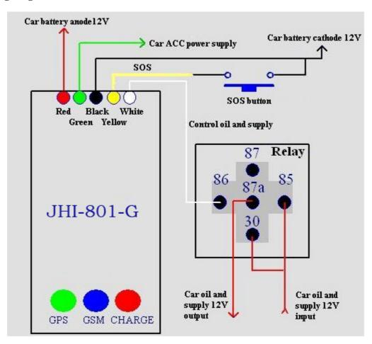
The external 5 wires of TLT-2H GPS/GSM tracker are as follows. Red for the 12V car power wire, connect to the car battery anode; Black for the earth GND, connect to the car battery cathode; Yellow for the SOS for help Control wire, connect external SOS switch button to car battery cathode; Green wire connect ACC car power supply, that is, with the car CD, radio, and other automotive electrical appliances in parallel. When the vehicle key puts in the ACC gear, the green
